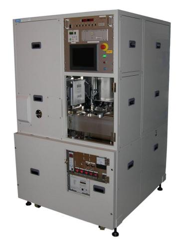
The SAMCO RIE-101iPH is a load-locked type inductively coupled (ICP) etching system. The system designed for R&D customers who require a flexible system capable of etching a large number of materials in one system.
