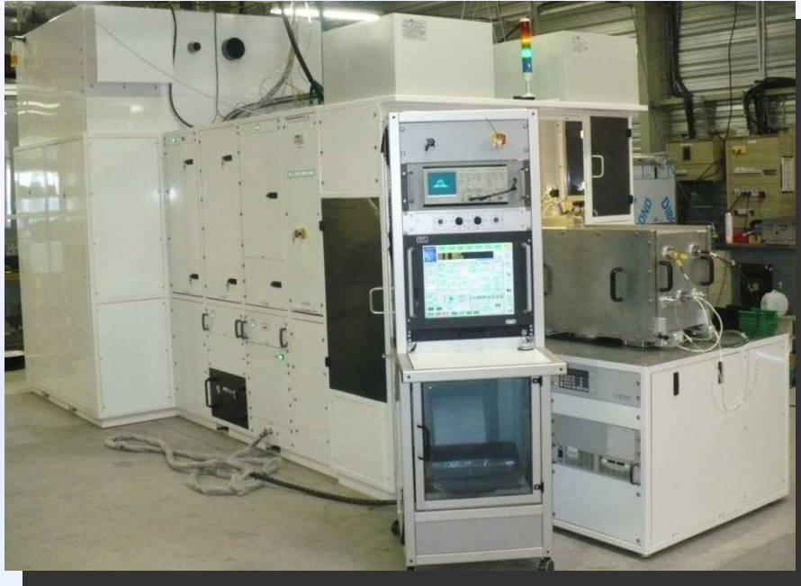
IMC 210RD v6 (NV4206 based) -Hot implant chamber extension -2 Gas Boxes with 1 liquid line
