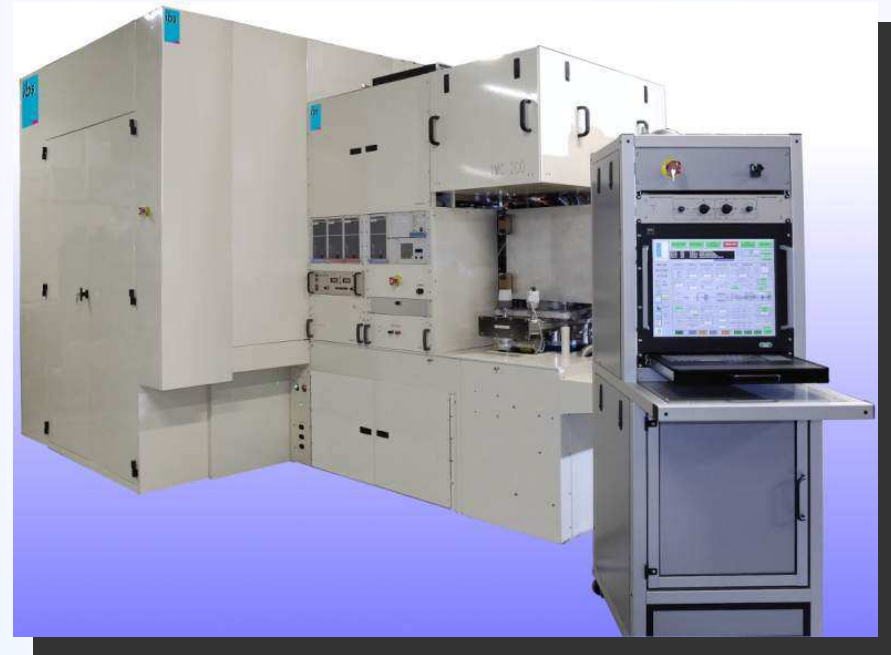
IMC 200RD v5 (CF3000 based) -Multi-platen configuration -Silicon coated beam line
